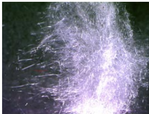
Photo 12: Mineral Wool Fibres (x10). Transparent, colorless to brown, isotropic, smooth cylinders straight or gently curved.
